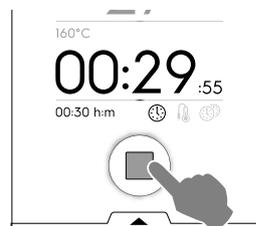
3. At the end of the cycle acoustic signals sounds A pop-up window opens showing the summary of consumption, time cycle and utility used.
