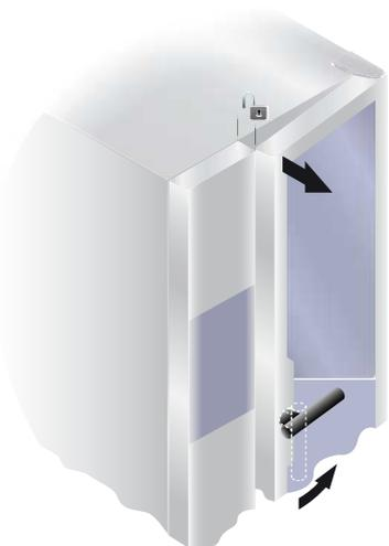
1. Rotate the handle by 90° counterclockwise to open the door completely. The cooking programme is stopped, if in progress.
