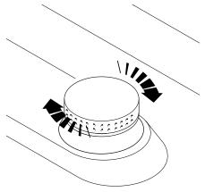
• Before lighting the burners make sure the flame spreaders are turned to the stop position.
