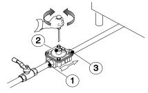
**NOTE!** These models are designed and certified for use with natural or propane gas. For natural gas, the pressure regulator on the header is set to 8" w.c. (20mbar).
