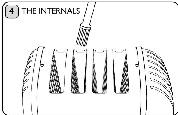
With the toaster unplugged from the power supply use a **SOFT BRUSH** to clean inside your toaster, do not use a sharp or metal utensil! Crumbs should be carefully brushed off the elements using only a soft brush, the toaster can be turned upside down and excess crumbs be shaken out.
