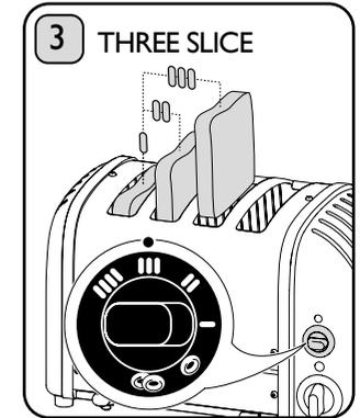
**4 slot model:** Select the three slice indicator. The three slots from the left will toast on both sides.
