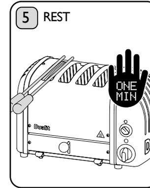
Allow to rest for a further minute inside the toaster to allow fillings to fully warm. **If neon light remains illuminated after use immediately isolate the toaster & call the service centre.**
