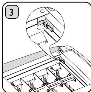
The fuse can be located in the rear corner of the toaster body.
