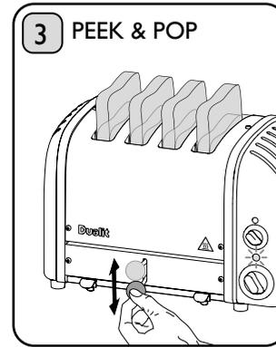
Check the progress of your toast at any time by pushing down on the 'ejector knob'. **If you remove your toast before the cycle is complete, cancel timer and unplug.**
