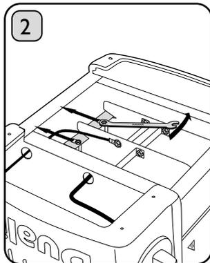
Loosen locking nuts on retaining plate using a 6.5mm spanner and slide back. **Ensure that the retaining plate is correctly in position when reassembling.**
