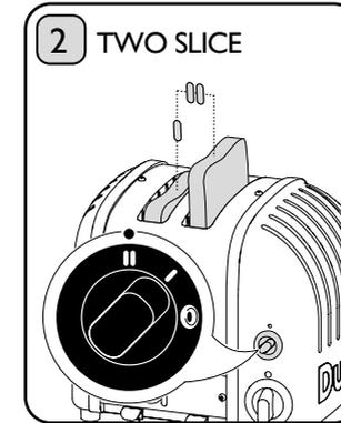
**2 & 4 slot models:** Select the two slice indicator. The two slots from the left will toast on both sides.
