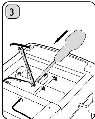
Unscrew brass links and wires.
