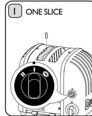
**2 & 4 slot models:** Select the one slice indicator on the 'selector switch'. The left hand slot will heat up on both sides.
