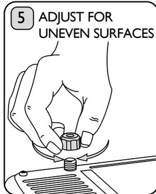
Your toaster is fitted with one adjustable foot which may be raised or lowered to compensate for uneven surfaces. The adjustable foot is located on the base of the toaster and is hexagonal in shape; rotate it to adjust the height.
