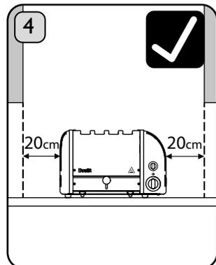
Place the toaster on an open level surface. Ensure the toaster is positioned at least **20CM CLEAR FROM ANY OVERHANGING CUPBOARDS, WALLS OR CEILING AND BEHIND TOASTER.**
