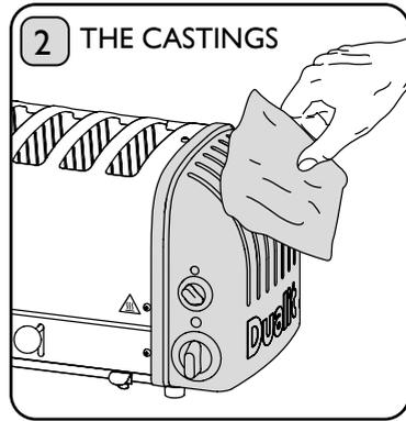
Wipe the aluminium end castings with a damp cloth. Do not use a chemical or abrasive cleaner.
