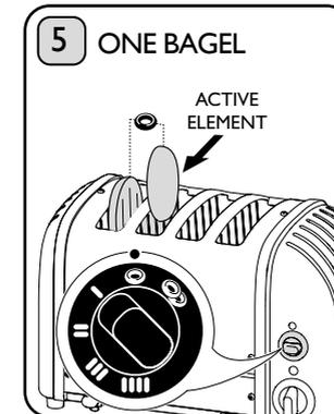
**2 & 4 slot models:** Select the one bagel symbol. Only the second element from the left will heat up.
