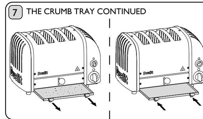
Crumbs will accumulate in the crumb tray and could catch fire if the tray is not emptied frequently. Pull out the crumb tray and wipe clean using a damp cloth. **CRUMB TRAY MUST BE IN PLACE BEFORE TURNING ON THE TOASTER AND DURING TOASTING.**
