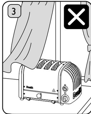
**DO NOT STORE OR USE YOUR TOASTER CLOSE TO CURTAINS OR FLAMMABLE MATERIAL.** A fire may occur if incorrectly positioned.
