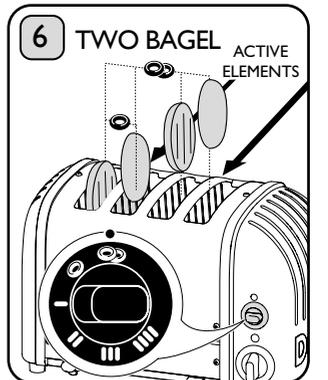
**4 slot models:** Select the two bagel symbol. Only the second and fourth element from the left will heat up.
