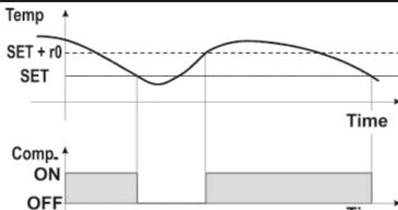
In case of fault in the thermostat probe the start and stop of the compressor are timed through parameters "Cy" and "Cn".
