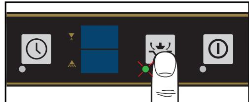
↳ During pump out, the Drain key LED flashes.
