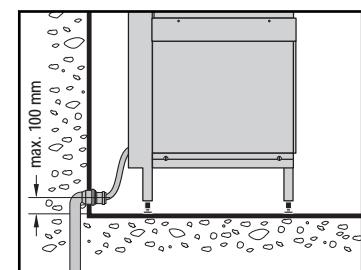
For these machine types, a floor drain is mandatory. Otherwise, residual water may remain in the tank and hose.
