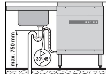
The connection between machine and site drain must not exceed the max. height of 0.75 m.
