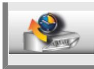
Press the **Shut-off delay of condensation hood** button and adjust the shut-off delay time for your condensation hood (1 min. – 30 min.) using the central dial.
