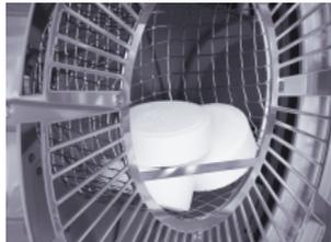
Insert the cleaning tabs into the indentation in the air baffle.
