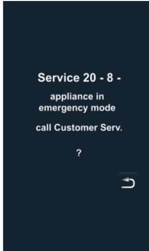
Faults on your unit which allow you to carry on cooking can be suppressed by pressing the "back" button.
