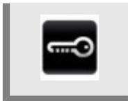
The key lock is deactivated by pressing the key for a further 3 seconds.
