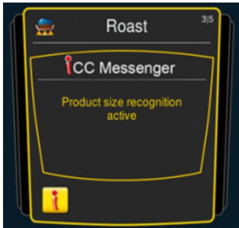
The iCC Messenger actively notifies you of processes and adjustments that iCookingControl performs. The iCC Messenger disappears automatically after 4 seconds.
