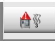
Press the **3 button**. **Cooking warning: Process interrupted** and use the central dial to set the time until the warning for the aborted cooking process on or off (5 sec. – 180 sec.; off).
