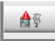
Press the **2 button**. **Cooking warning: Check the product** and use the central dial to set the time until the warning is emitted on or off (5 sec. – 180 sec.; off).
