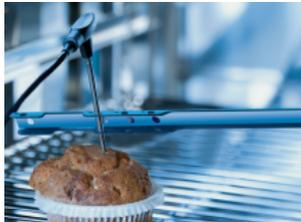
Use the positioning aid if the core temperature probe could fall out of the food (for instance if the food to be cooked is of a soft consistency or not very thick).
