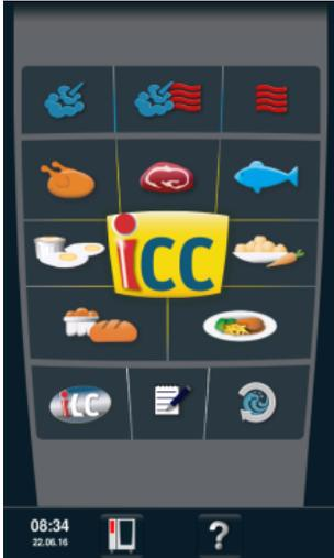
You can access the **iCookingControl mode** by selecting your required results, for example by selecting poultry, side dishes or fish. See the iCookingControl mode section for a description.
