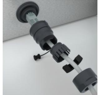
Thread the individual components on the cable, as shown in the diagram. Then plug the LAN cable into the socket.
