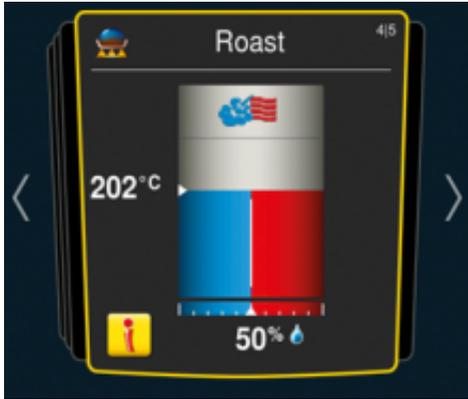
The i button appears as soon as a decision was made or a setting is being adjusted in the background. Press the i button or press the central dial to open the iCC Monitor in the iCC cockpit.
