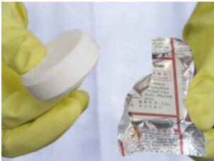
Cleaning tab: Remove protective film.
