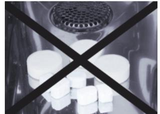
Do not insert tabs into the cooking chamber - risk of damage.
