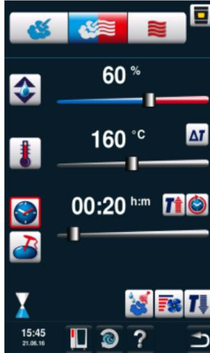
You enter the **Combi-steamer mode** by pressing the button “steam”, “combination” or “convection”. See the Combi-steamer mode section for a description.
