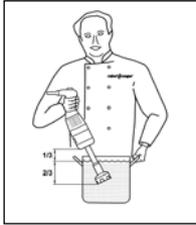
Always make sure that the bell is sufficiently immersed to avoid splashing and that the air vents of the motor unit does not come into contact with any liquid.
