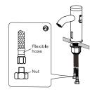
As the picture 3 shown, put the filter in the angle valve and use the spanner to connect the flexible hose to the angle valve.
