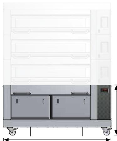
The height of the proofer without the bottom section and castors is 560/740 mm. With the bottom section and castors, the dimensions are 810/990 mm.
